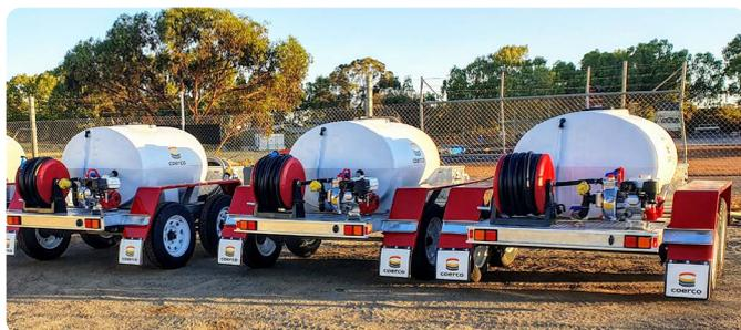
The design incorporates a tandem axle that has been designed to maximise stability and weight distribution for easy access to differing terrains like sand and gravel, and easy maneuverability in urban areas.
